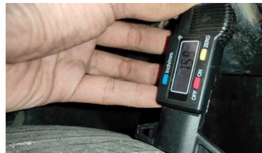
Cek Ketebalan Ban Belakang Kiri
